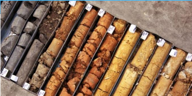
Core cutting from a field investigation
