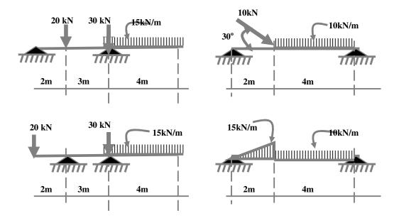
5) Calculate the reaction and its direction for the two staircase sections shown below
