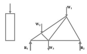
*Examples of Applications* Column loads Reactions from end of beams Loads at nodes of frameworks
