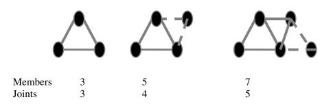
Figure 2. 5 Statically determinate pin jointed frameworks
