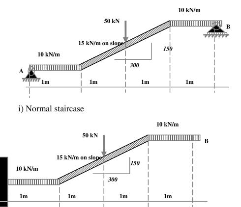
ii) Fixed on one side staircase (cantilevering)
