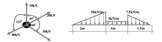
4) Calculate the reaction and its direction at A for a post loaded with point loads at different angles as shown below
