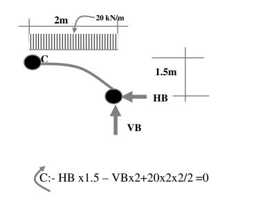
From equation 3 and 4:- 8VB+400 = 0 VB = 50kNHB=60/1.5 =40kN From equation 1:- VA + 50= 120:- VA =70kN From equation 2 HA = HB =40kN
