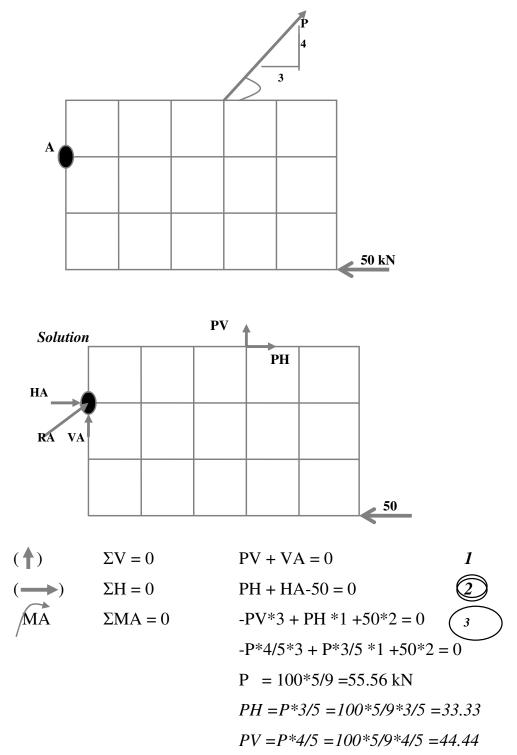
(1) P\*4/5 +VA = 0 VA =-P\*5/4 =-100\*5/9\*4/5 =-44.44kN P\*3/5 +HA -50 = 0 HA =50- P\*3/5 = 50-100\*5/9\*3/5 = 16.67 kN 16.67 kN16.67 kN
