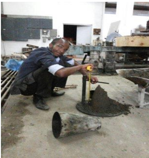
Plate 3- 1: Measurement of amount of slump
