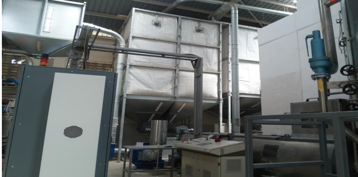
Plate 2- 7: Silos and other machinery used for manufacture of polystyrene (National Housing Corporation)
