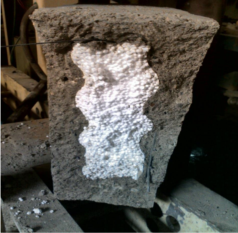
Plate 4- 6: Expanded polystyrene wall panel intact after failure under compression load
