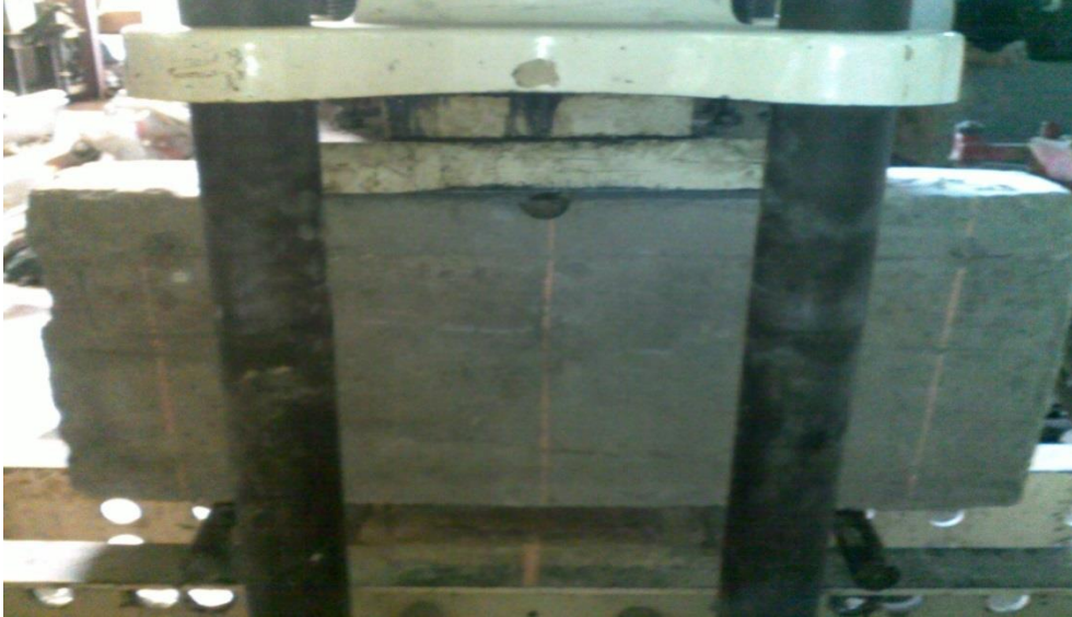
Plate 4- 4: Wall panel under flexural loading
