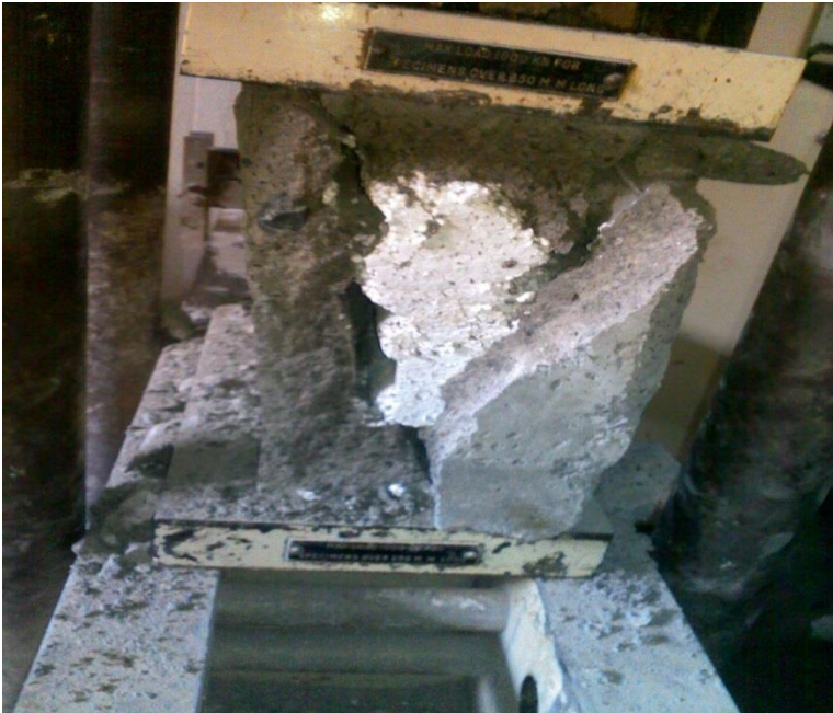
Plate 4- 7: Failure of wall panel under compressive load
