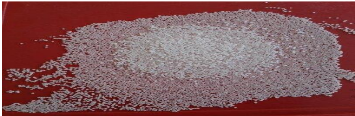
Plate 2- 3: Pre-expanded polystyrene beads (Foam technology (2013))
