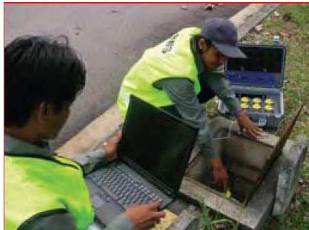
Figure 2.10: A computerised noise logger in use (Farley, 2008)
