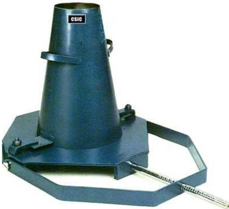
**Figure 1: Slump Test Apparatus**
