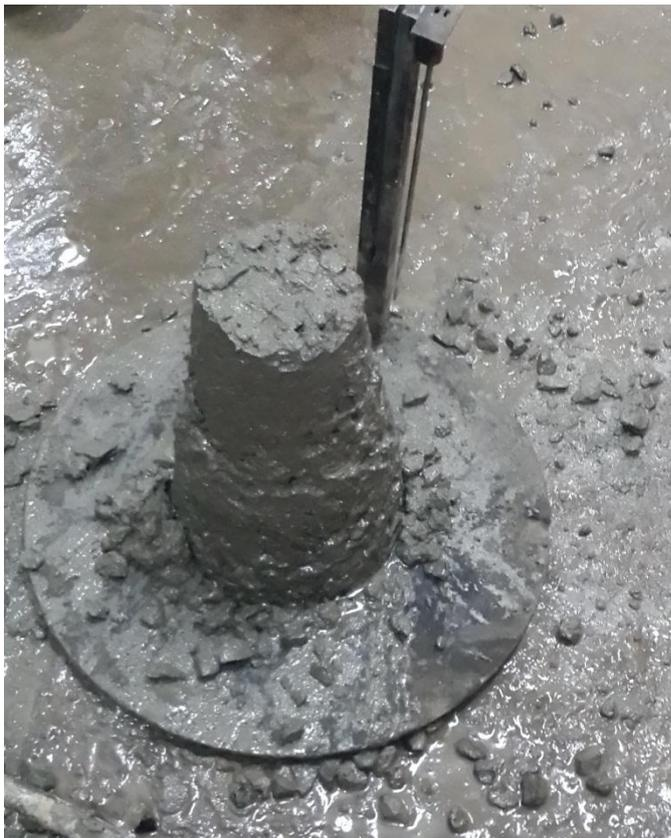
**Figure 2: Slump Test**
