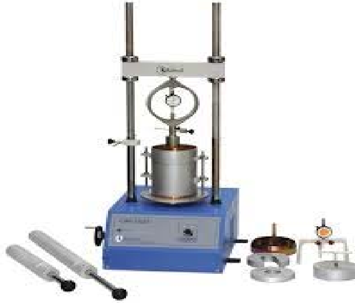
Figure 7:A CBR setup ( www.mandava.ac.in )
