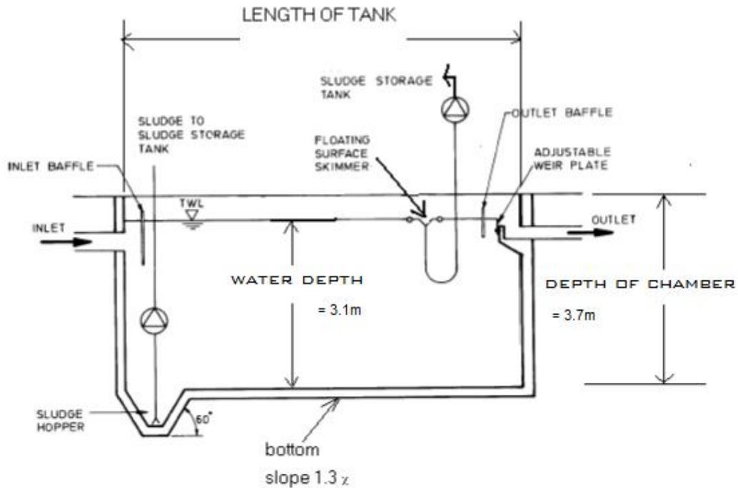
Fig. 4: Primary Sedimentation Tank
