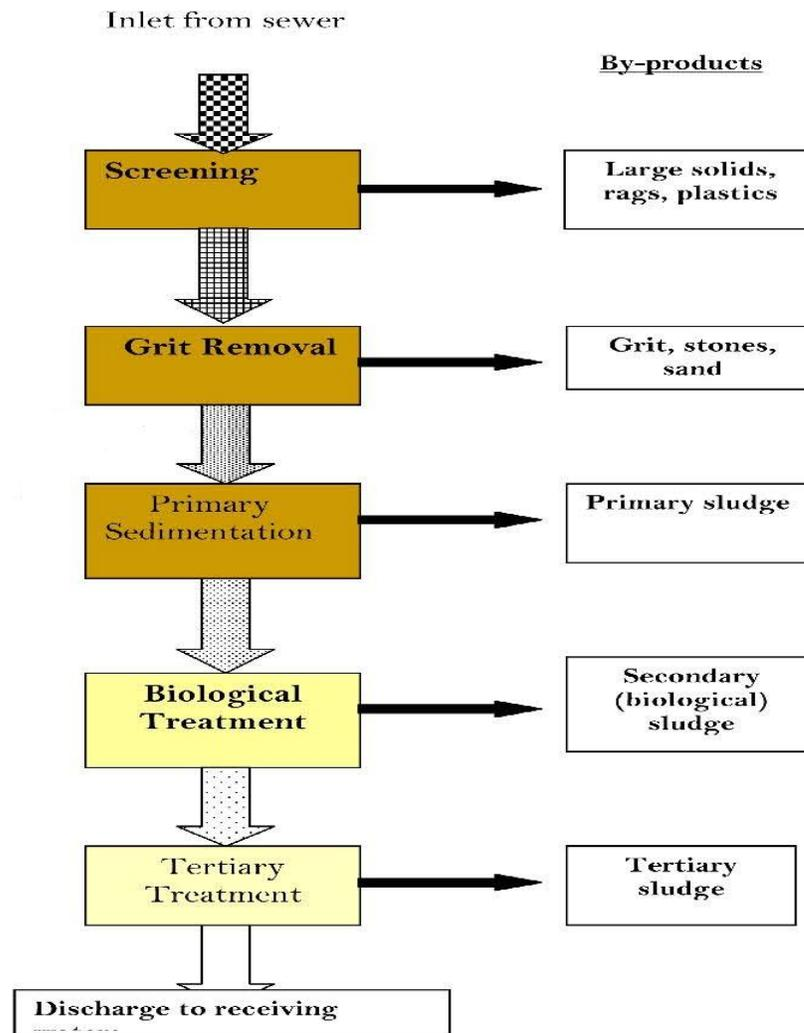
*Fig. 1: Flow chart for wastewater treatment process*
