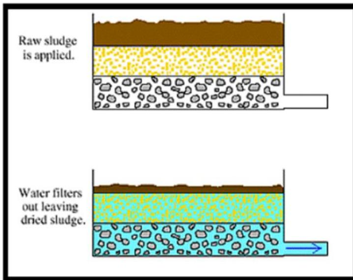
*Fig 2: Sludge drying bed*
