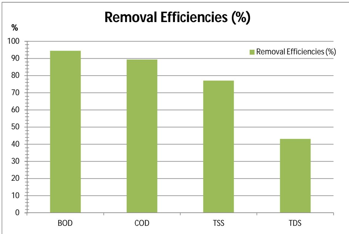
**Figure 4.4: Graphical Representation of Removal Efficiencies (Kabete Flats)**
