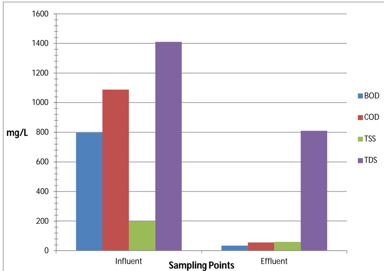
**Figure 4.1: Average of different parameters in the ETP (Maasai Mall)**
