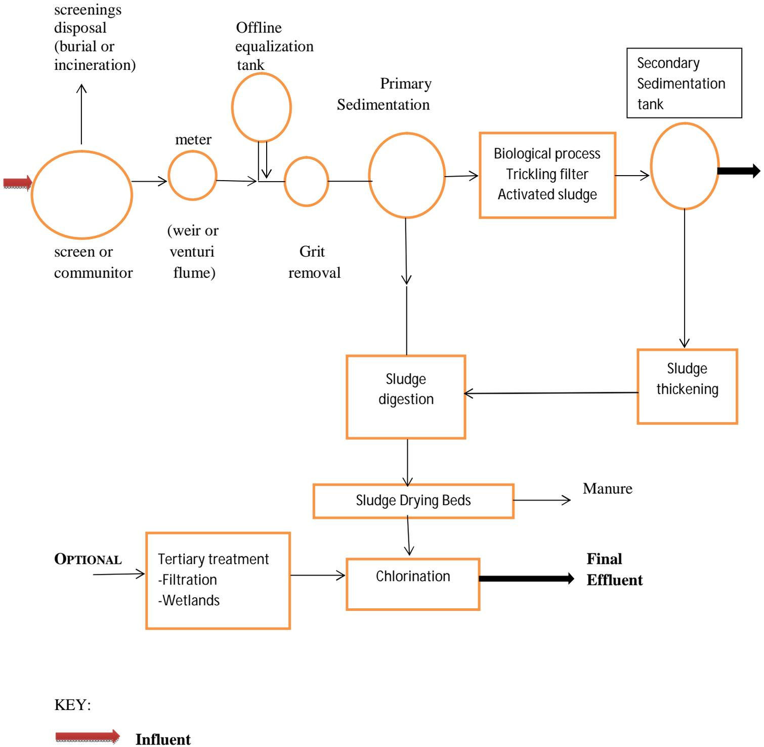
**Figure 2.1: Typical Flow sheet of a Conventional Treatment Plant**
