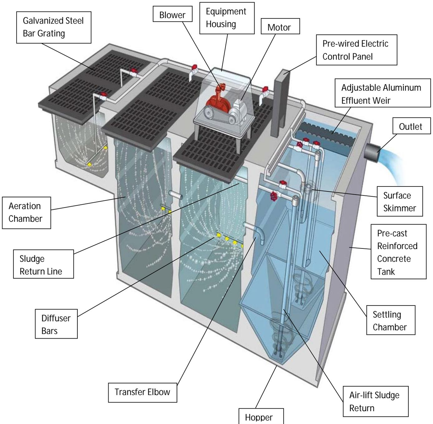
**Figure 2.2: Cut-away of a Typical *JET Inc.*<sup>®</sup> Commercial Wastewater Treatment Plant**
