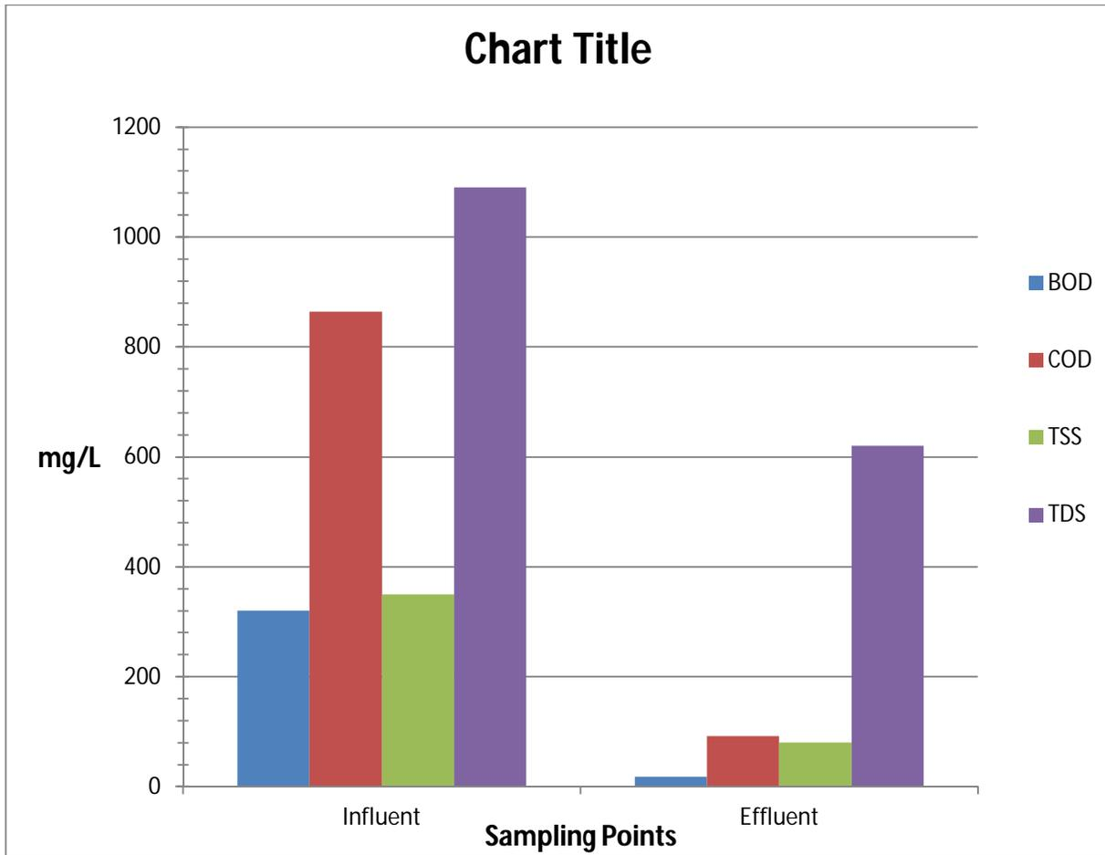
**Figure 4.3: Average of different parameters in the ETP (Kabete Flats)**
