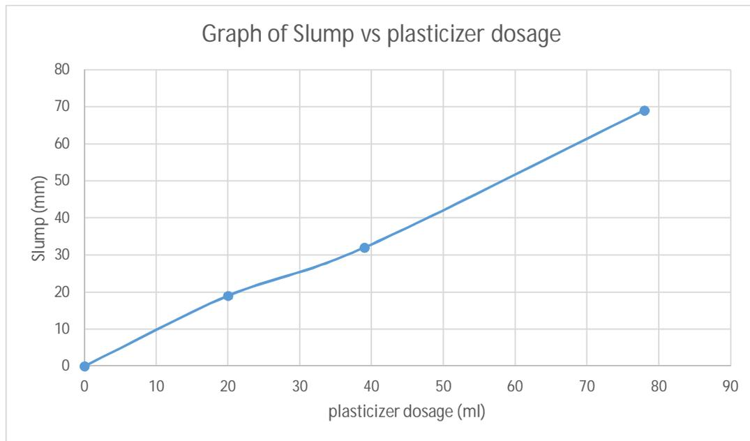
Figure 6. Graph of Slump vs Plasticizer dosage.
