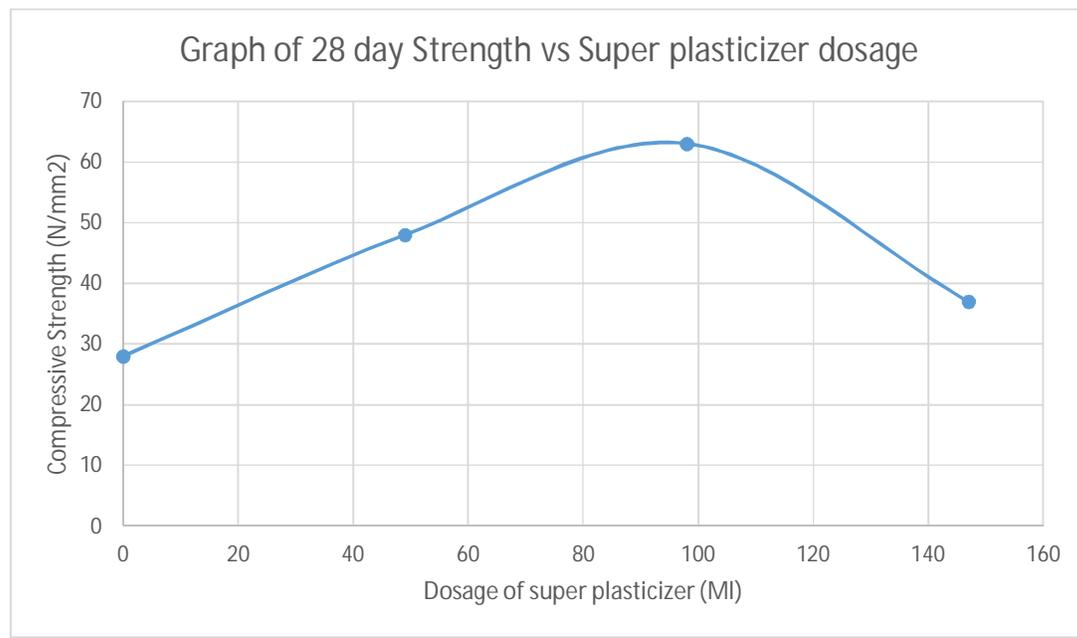
Figure 9. Graph of 28 day strength vs Super plasticizer Dosage
