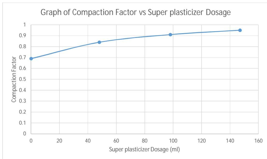
Figure 7. Graph of Compaction Factor Vs Super plasticizer Dosage
