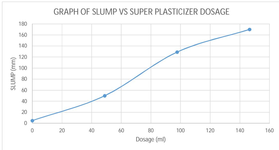
Figure 3. Graph of slump vs Super plasticizer
