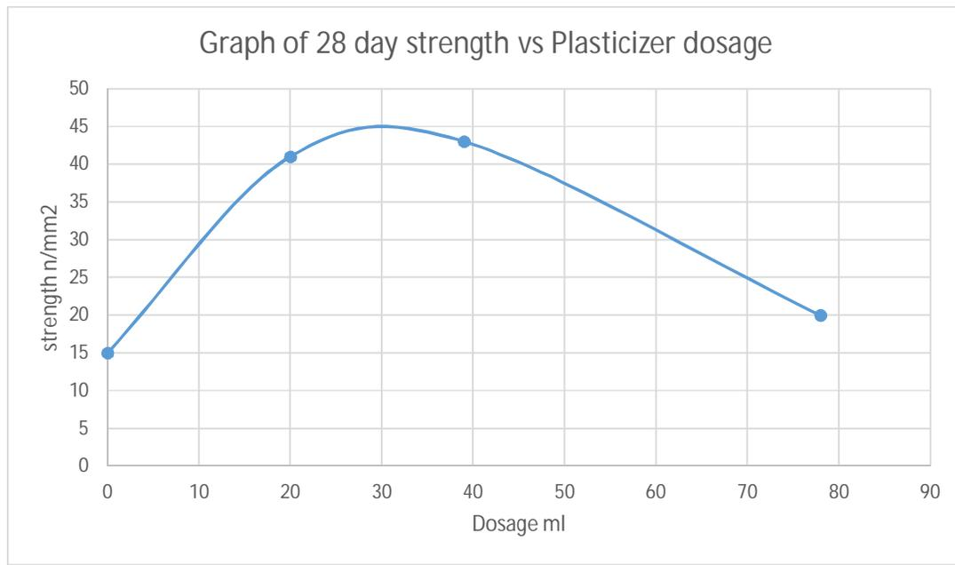
Figure 11. Graph of 28 day strength vs Plasticizer Dosage
