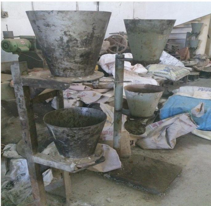
Figure 1. Compaction factor apparatus
