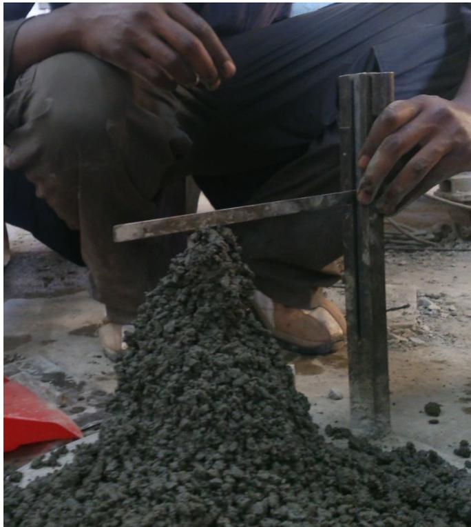
Figure 5. Concrete mix with Super plasticizer added showing shear slump
