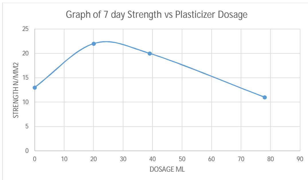
Figure 10. Graph of 7 day strength vs Plasticizer Dosage.
