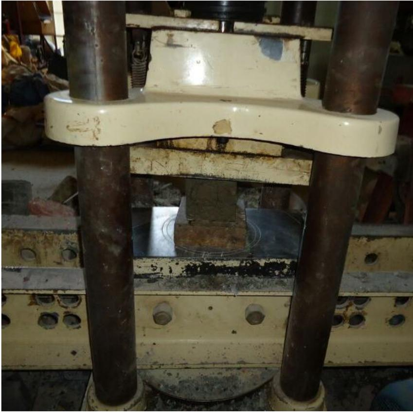
Figure 2. Compression testing machine.
