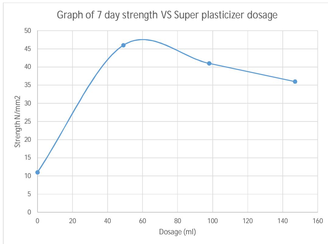
Figure 8. Graph of 7 day strength vs Super plasticizer dosage
