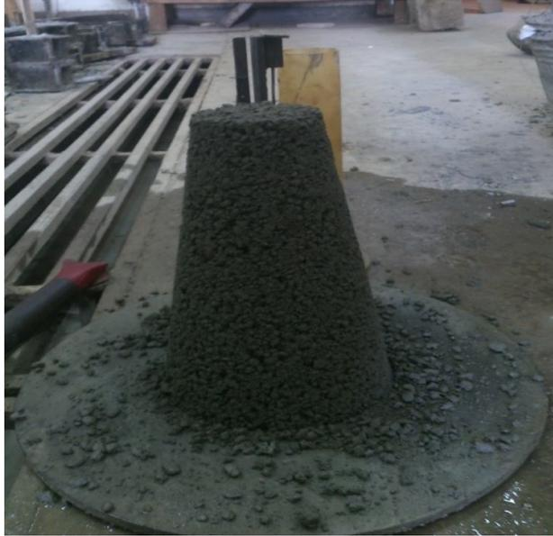
Figure 4. control mix with No super plasticizer added showing normal slump
