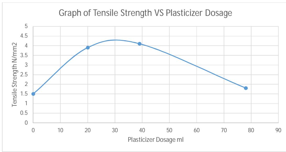
Figure 14. Graph of Tensile Strength vs Plasticizer Dosage
