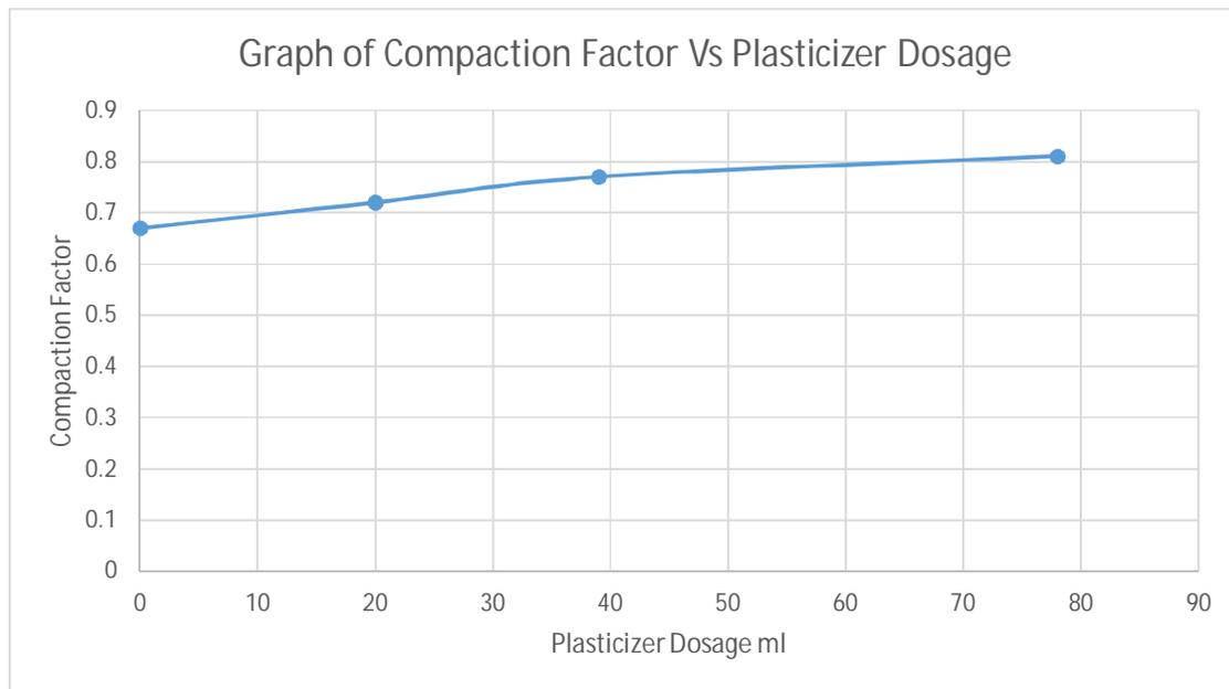
Figure 8. Graph of Compaction Factor vs Plasticizer Dosage.
