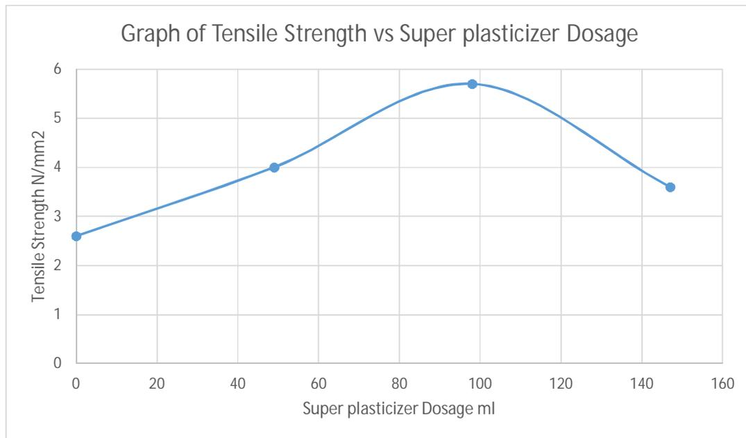
Figure 13. Graph of Tensile strength Vs Super plasticizer Dosage
